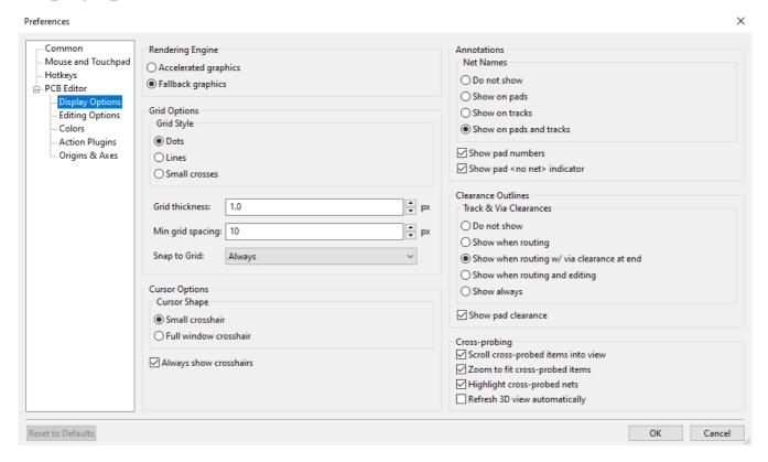
Rendering Engine: Controls if Accelerated graphics or Fallback graphics are used.
