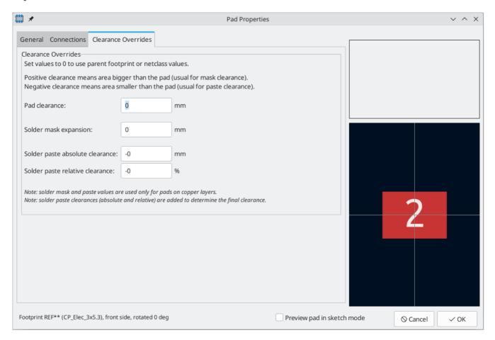
**Pad clearance** controls the minimum clearance between the pad and any copper shape (tracks, vias, pads, zones) on a different net. This value is normally set to 0 which will cause the pad clearance to be inherited from any clearance override set on the footprint, or the board's design rules and netclass rules if the footprint clearance is also set to 0.
