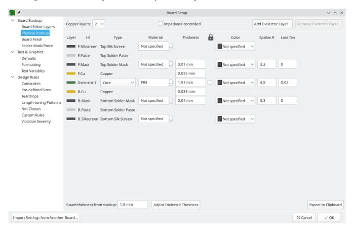
Set the number of copper layers in the upper left corner and then enter the physical parameters of the stackup if desired. These parameters may be left at their default values, but note that the board thickness value will be used when exporting a 3D model of the board, and layer thicknesses will be included in net length calculations for any nets that include vias. If you plan to use these features, it is a good idea to ensure that the stackup thickness is correct.
